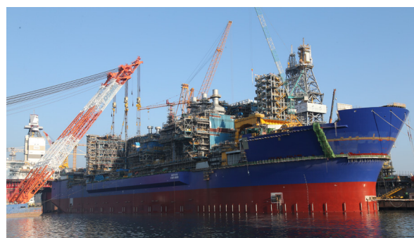
Figure 6: Ichthys FPSO under construction in Korea
